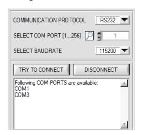
A click on the magnifier symbol in the **CONNECT** tab opens a list with all the possible **COM PORTS** in the display.
