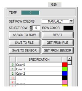
With SAVE TO SENSOR and GET FROM SENSOR the TABLE ATTRIBUTES can now be saved to the sensor and loaded from the sensor.
